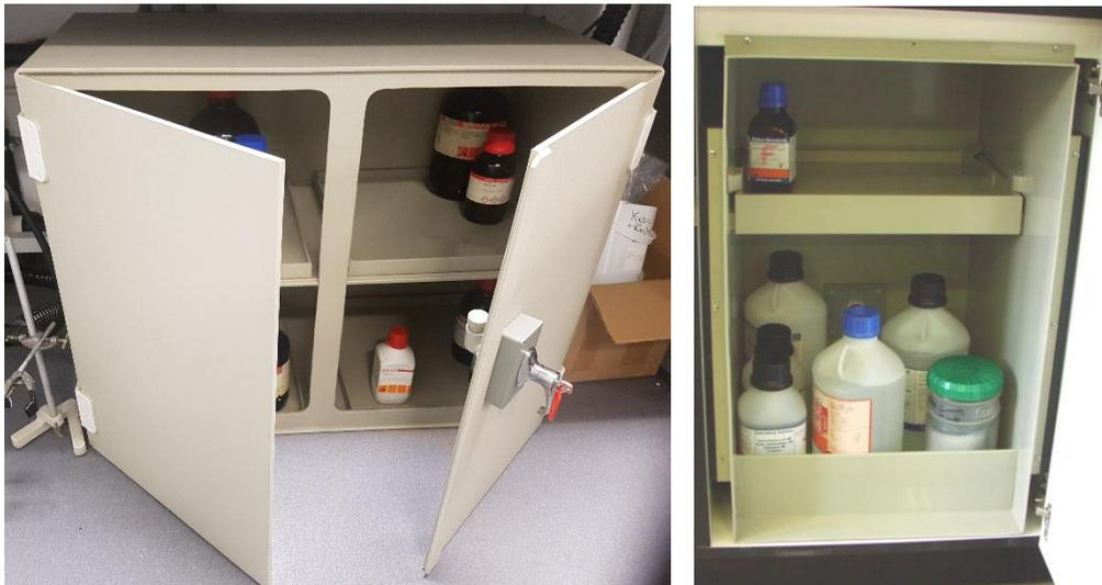
**Figure 2 – Bottles stored in drip trays within ventilated acids cabinet including example of chemically resistant secondary containment (BDH / VWR Safepak bottom right)**
