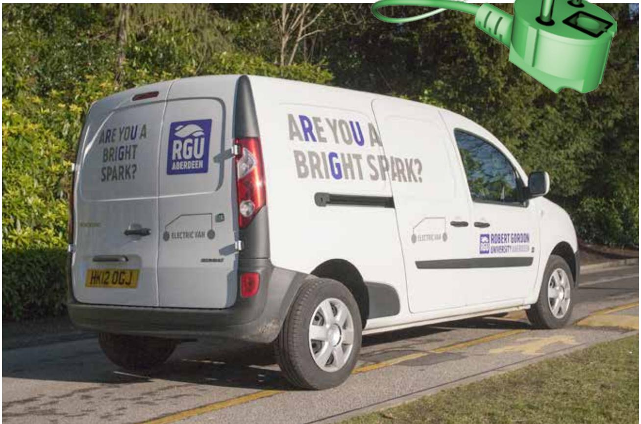
In order to reduce CO2 emissions and save costs, the University has leased an electric van which is currently being used as the Mailvan. The Renault Kangoo ZE can do approximately 70 miles on one charge, with low running costs. The initial lease is for 12 months, but is expected to continue at the end of the trial period.
